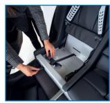
Tuck the harness out the way so nothing is restricting the Minimac locking into position.
