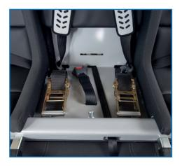
The tether straps are fastened into two ratchet adjusters which are situated under the seat cushions.
