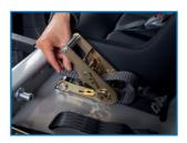
Push any loose tether strap back through the ratchet so it does not hang over the front of the Multimac.
