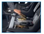
Check that the legs are pressed firmly to the floor and do not rattle.
