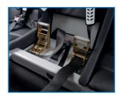
Ensure the straps are not twisted. Feed the tethers through the slot in the spindle. Slide the legs into their sockets.
