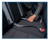
Tilt the Multimac forwards slightly to insert the tether straps through the holes in the back of the chassis.
